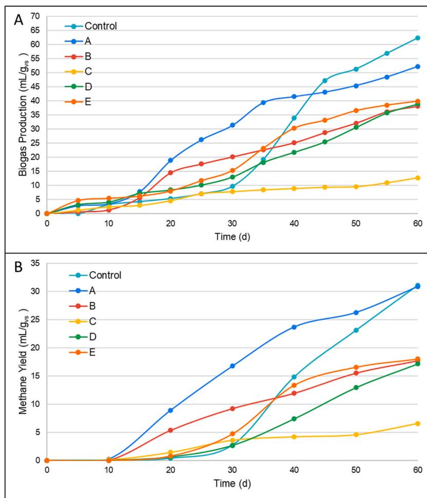
Fig. 5. A) Biogas production and B) methane yield for co-AD of SDCM with mixture of SW and PPM at different concentrations.
