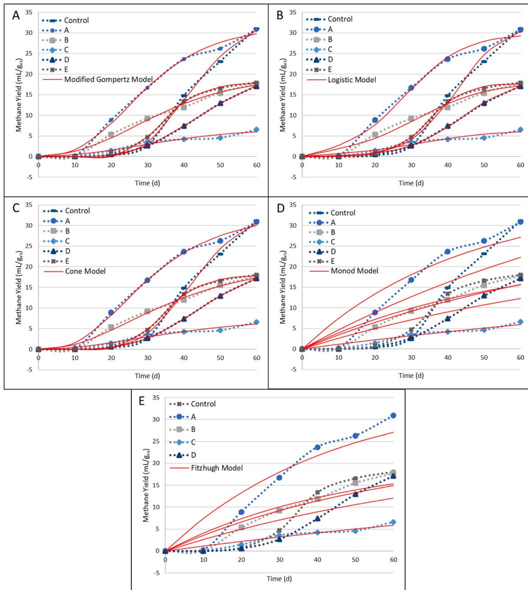
**Fig. 6.** Comparison of co-AD of SDCM with mixture of SW and PPM at different concentrations between the actual and predicted methane yield (A) Modified Gompertz model (B) Logistic model (C) Cone model (D) Monod model (E) Fitzhugh model.
