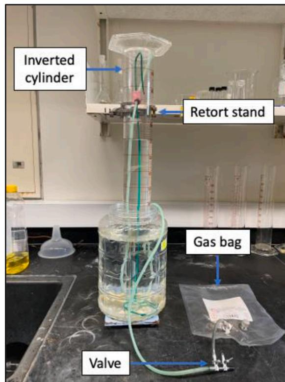
Fig. 1. Water displacement method.
