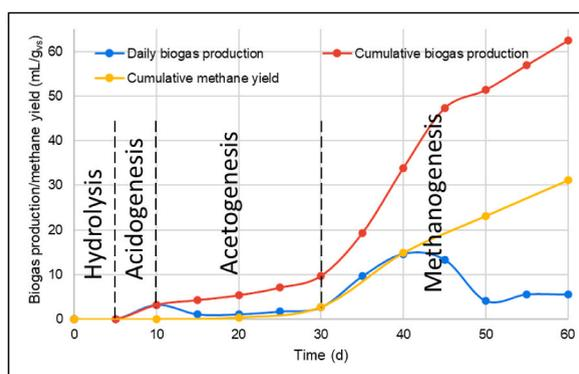
**Fig. 4.** Daily and cumulative biogas production and methane yield from co-AD of SDCM.
