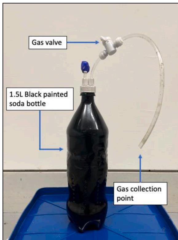
Fig. 2. Digester setup.
