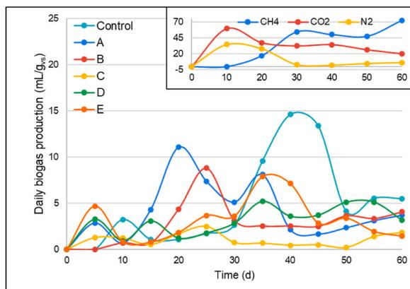
**Fig. 3.** Daily biogas production of co-AD of SDCM with mixture of SW and PPM at different concentrations (Inset picture: gas composition produced from Control).
