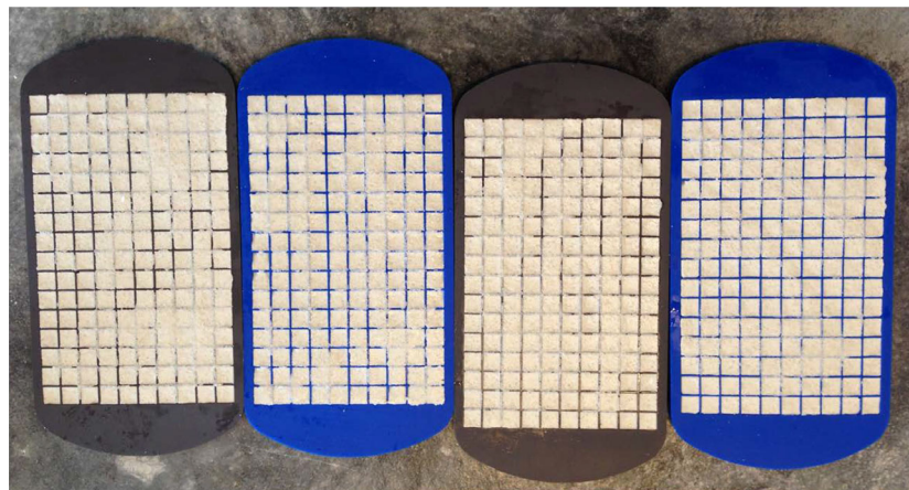
Figure 1 Production of standardized concrete coupons by filling 1-cm 3 silicone ice cube moulds with ready-mix concrete. Photo courtesy of Tod Barber, Reefball Inc., Nokomis, FL. [Colour figure can be viewed at wileyonlinelibrary.com ]
