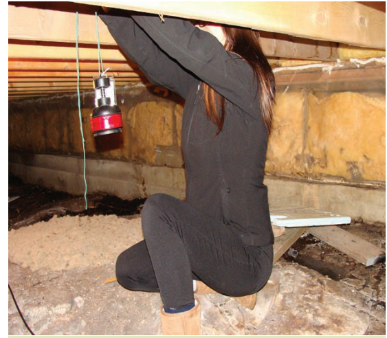
Figure 4: Hanging electret in a crawl space, under bedroom. The crawl space was made over bare rocks.
