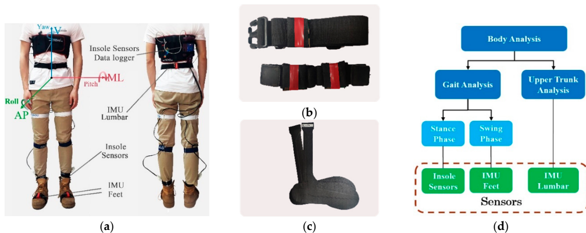
Figure 1. (a) Wearable sensors used in this experiment, including three inertial measurement unit (IMU) and a pair of insole sensors. Two IMU are attached to feet with elastic belt in the position that is closed to toe (IMU Feet). The other is attached to the low back, where it is closed to L3 region (IMU Lumbar). A pair of insole sensors are put into subject's own shoes and the data logger of insole sensors is fastened in the subject's body. In addition, mediolateral (ML), vertical (V), anterior-posterior (AP), Pitch, Roll and Yaw directions are shown. (b) Representation of three IMU with elastic belt. (c) A pair of insole sensors (Novel, Germany). (d) A diagram of human body analysis using insole sensors and IMU.
