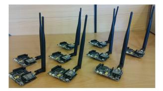
Figure 7. Waspmote devices equipped with BLE module.
