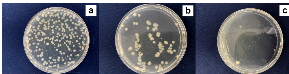
Figure 6. Visual bacterial cultures for undyed cotton fabric (a) and dyed cotton fabrics with 5% (b) and 10%owf (c) GSE.
