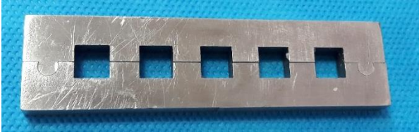
Fig. 1. The mold used for fabrication of composite blocks.
