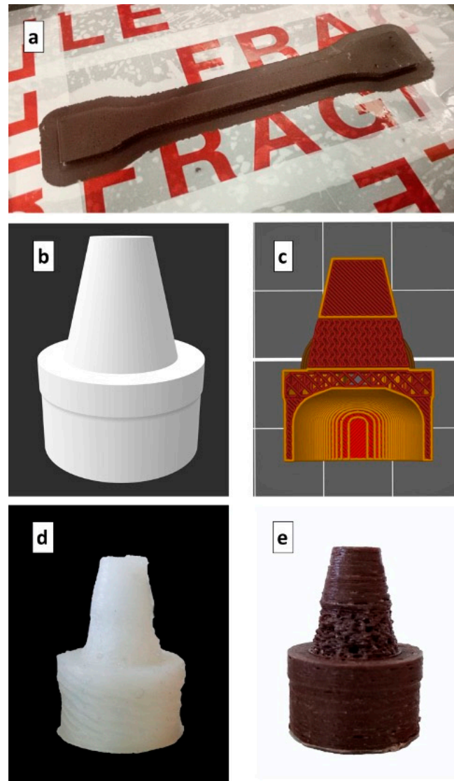
Figure 2. (a) Tensile specimen printed with the pozzolan composite. (b) 3D model of the prototype for precision irrigation. (c) Longitudinal section of the sliced prototype. (d) Prototype sample 3D printed with neat HDPE. (e) Prototype sample 3D printed with composite at 20% pozzolan.
