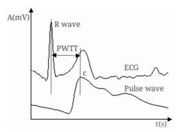
Fig. 1. PWTT measurement from ECG and pulse wave signals.
