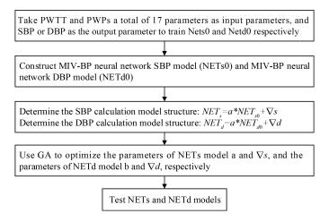
Fig. 3. Flow chart of the non-invasive continuous blood pressure measurement models based on the GA-MIV-BP neural network.
