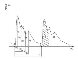
Fig. 2. Time domain characteristic parameters of pulse wave.
