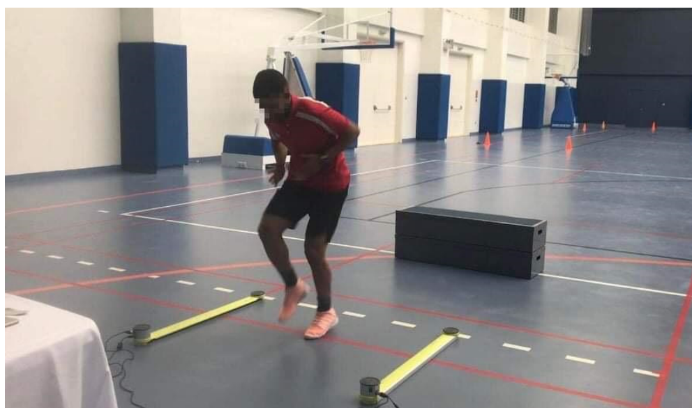
Figure 2. TAP test. In standing up position, the players are asked to tap the feet as quickly as possible on the ground with two alternating limbs for 4 s using Optojump Next (Microgate Next, Bolzano, Italy).
