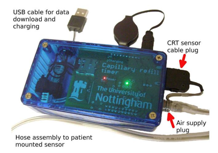
**Figure 7.** The CRT data-logger, assembled view.
