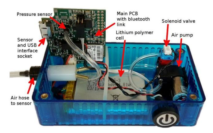
**Figure 3.** The CRT data-logger base unit, partially assembled view.
