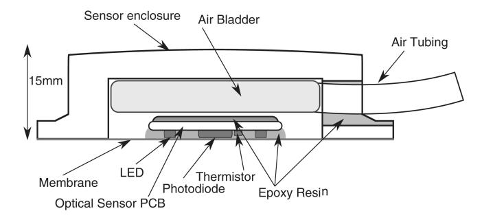
**Figure 1.**Cross sectional diagram of sensor construction. A thermistor was mounted to the skin facing side of the PCB, allowing approximate skin surface temperature measurement.
