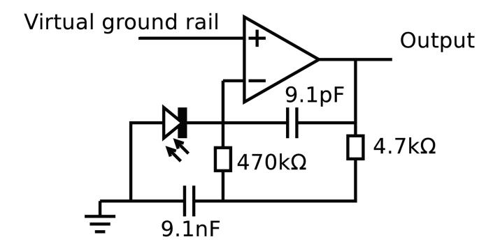
**Figure 5.**Single op-amp photodiode amplifier, designed using optimisation in SPICE package (virtual ground is held at 1.26 V).
