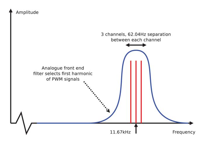
**Figure 4.**Schematic of the frequency division scheme adopted for use with the CRT datalogger device.
