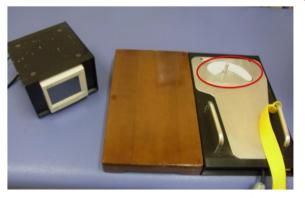
Fig. 1 Push-type toe-grip strength meter. Toes press the floor, facing the strain gauge installed in the cantilever (red circle)
