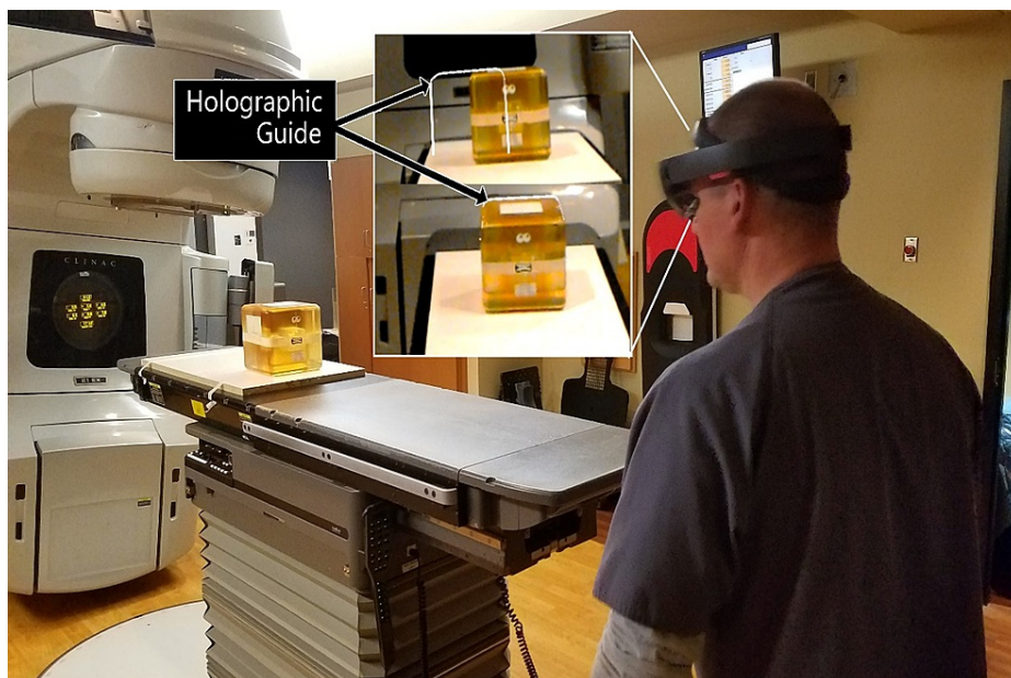
FIGURE 2: A therapist adjusts the couch positions to align a physical phantom to a holographic outline, visible to the user as a 3D glowing cube, using the Microsoft HoloLens. The top image shows that the current alignment is off, and the lower image shows a perfectly aligned phantom.
