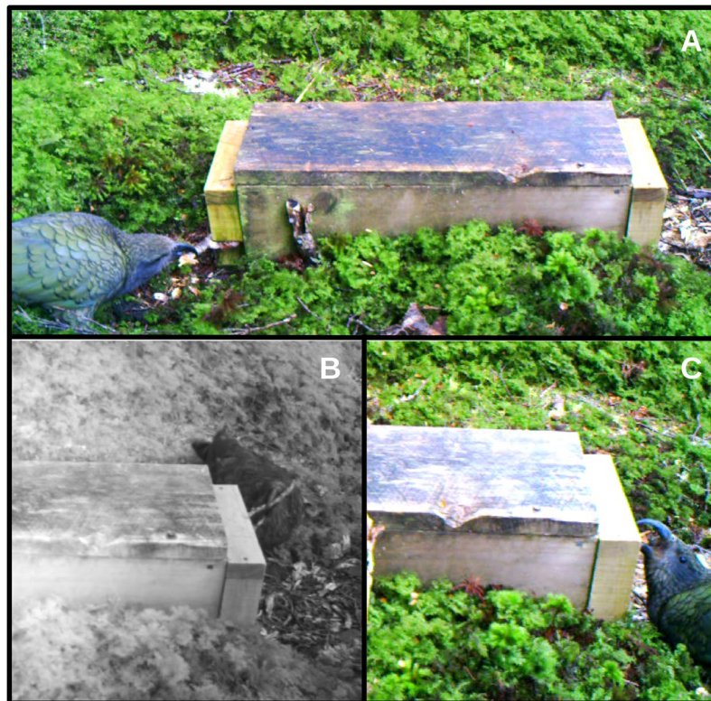
Figure 4. Frames from the Supplementary video footage showing the kea tampering with trap-box LC02. (A) The kea probing with a stick in the visible side entrance (Video S1). The lighter-coloured wood on the ends of the trap-box are modifications to move the entrances from the ends to the sides of the unit to try and prevent kea setting off snap-traps inside. (B) The kea probing with a stick in the side entrance on the opposite side of the trap-box (Video S4). The footage was taken in infrared because of low light conditions. (C) The kea biting trap-box LC02 (Video S3).
