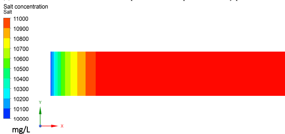
(a) Salt concentration distribution in the presence of the spacer on the x-y plane where z = 0.41 mm.
