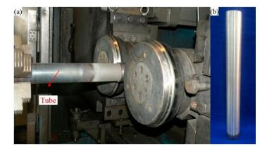
Figure 1. (a) Double-wheel spinning installation and (b) as-spun tube.
