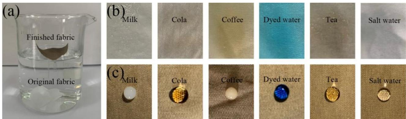
**Figure 9.** (a) The water soaking phenomenon of the original fabric and the superhydrophobic fabric, (b) the state of different droplets on the original fabric, and (c) the state of different droplets on the superhydrophobic fabric.
