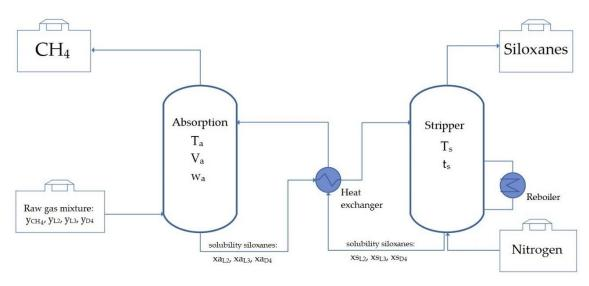
Figure 1. Simplified process flow diagram of siloxanes separation using deep eutectic solvent (DES).
