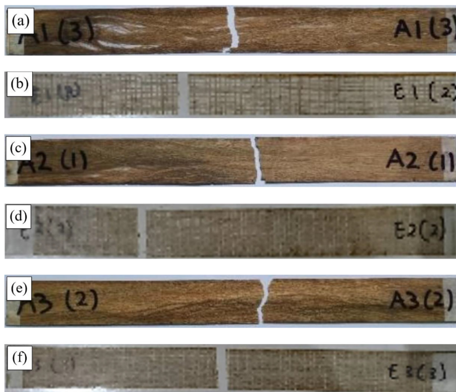
Figure 7. Fracture specimens (a) 15 % unidirectional WH fiber composite. (b) 15 % WH woven fiber composite (c) 25 % unidirectional WH fiber composite (d) 25 % WH woven fiber composite (e) 35 % unidirectional WH fiber composite (f) 35 % WH woven fiber composite.
