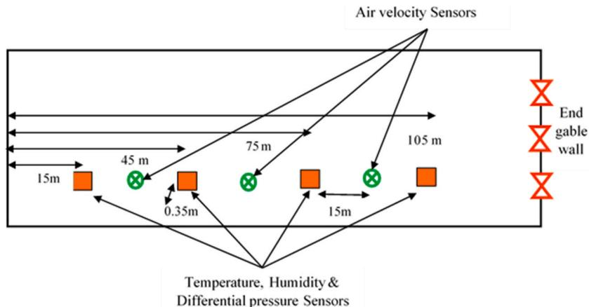
Fig. 3. Schematic drawing sensors location in the broiler house.
