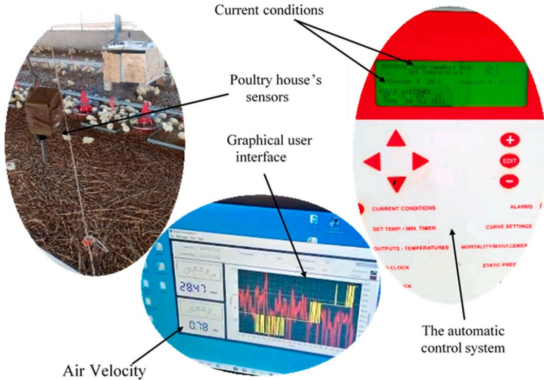
Fig. 4. Illustration of different components used in monitoring system.
