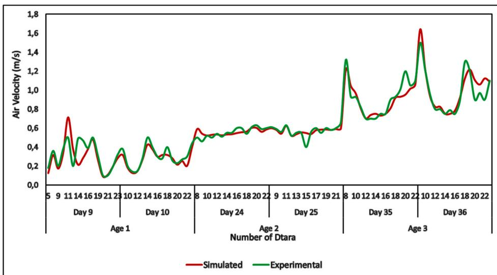
Fig. 5. Simulation of the inside air velocity compared to the experienced measurements.
