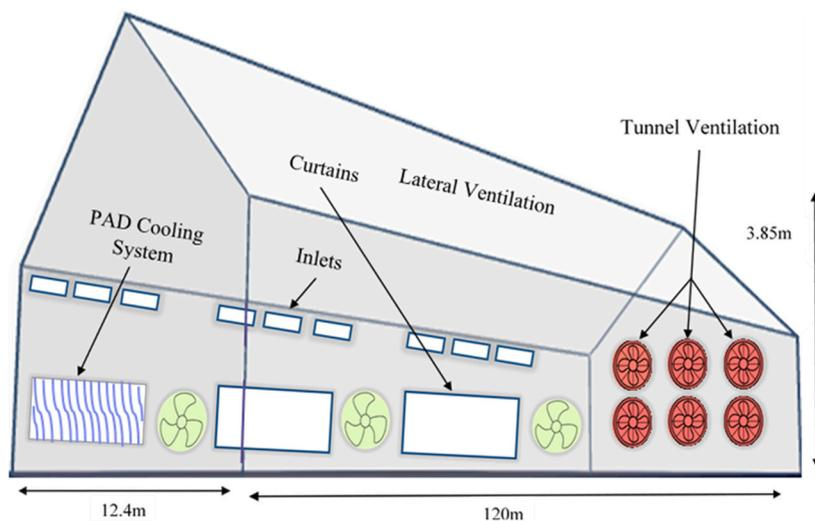
Fig. 1. Schematic drawing of the broilers house's: left view.
