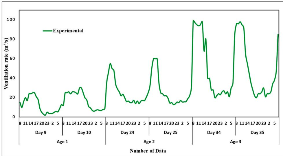
Fig. 8. Monitored ventilation rate variation during the rearing period.
