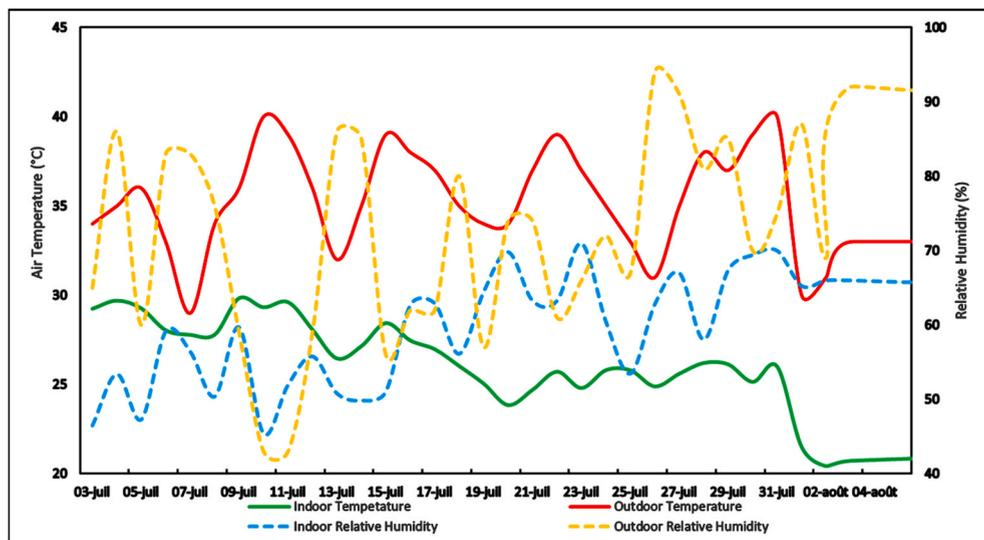
Fig. 7. Monitored indoor and outdoor air temperature and relative humidity.
