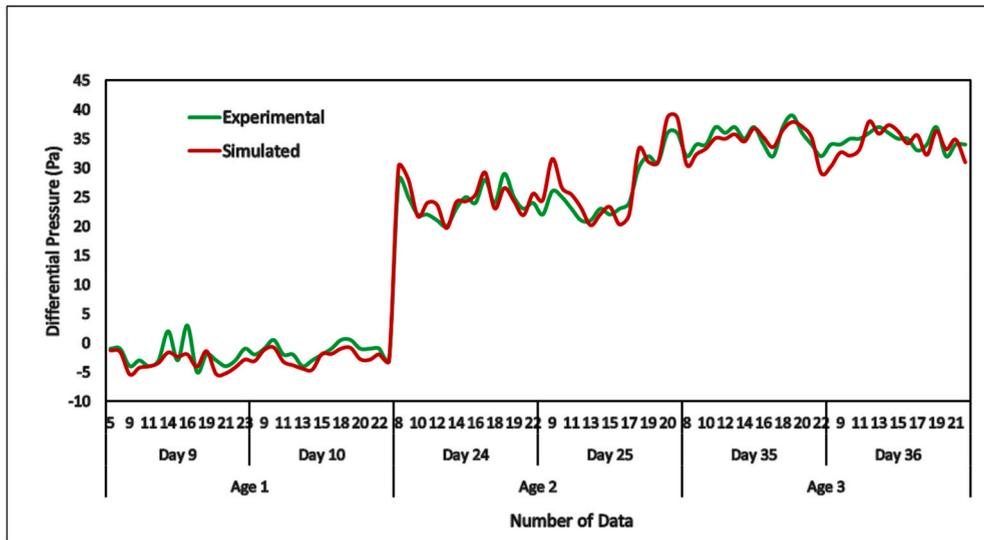
Fig. 6. Simulation of the differential pressure compared to the experienced measurements.
