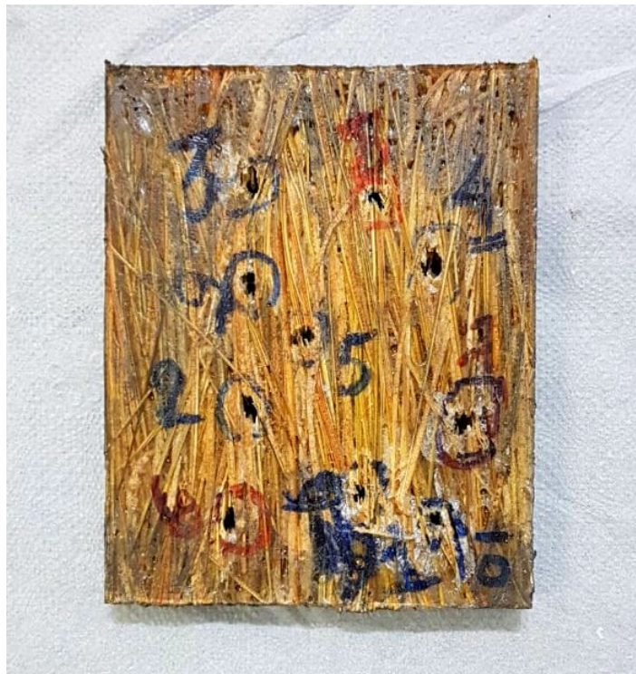
Figure 7. Target subjected to ballistic impact 30 vol% epoxy-caranan fibers composites.
