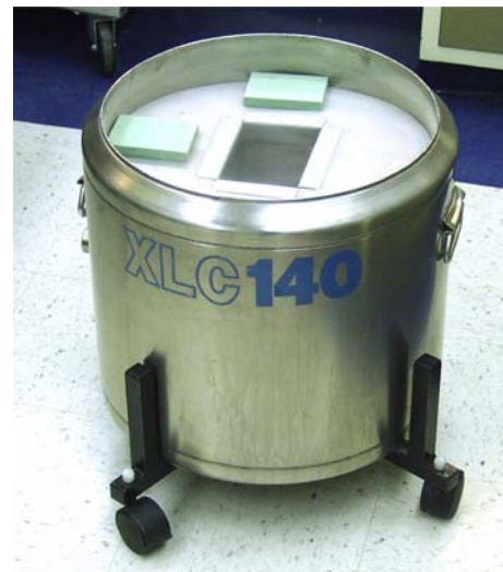
Fig. 13 Vessel model XLC140, and a pair of Teflon-coated aluminum plates. A pair of Teflon-coated, aluminum plates (each plate measuring 1.0 \times 8.0 \times 10.0 cm) for freezing blocks of tissue, rest on the shoulder of the double-walled vacuum vessel XLC140 (XLC140 vessel provider (8/2002): LNV Freezing Vessel, MVE, Inc., Two Appletree Square, Suite 100, 8011 34th Avenue South, Bloomington, MN 55425-1636. Phone: 1-800-2474446, ask for Steve Shaw, Sales Manager. XLC140 vessel with plain lid cover, foam insulation, vapor shipper insert, and castor wheelbase. Ask for Harvard BTRC specifications.)
