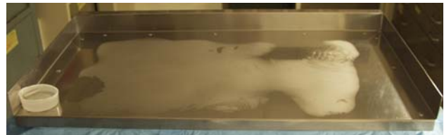
Fig. 11 The cold surface consists of a Styrofoam platform on a mobile cart, which is overlaid by a carpet of ice packs wrapped with a cotton towel on top of which a steel plate is placed. The space between the ice packs and the steel plate can be adjusted to control the temperature of the plate. On the cold steel plate, the coronal slices of the cerebral hemisphere are laid down with the posterior aspect facing up. The container on the left corner of the steel plate holds absolute ethyl alcohol and a razor blade for harvesting blocks from the coronal slices
