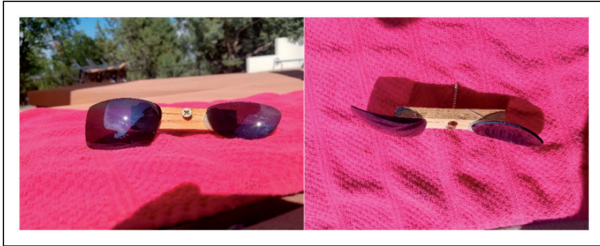
Figure 3. Sunglass lenses attached to a short stick in opposite orientations.
