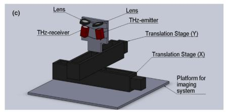
**Figure 1.** (a) Terahertz setup design. (b) Photograph of the setup once assembled while being tested. (c) Schematic representation of the raster-scanning imaging array which is placed on the platform under the windows as indicated in (a).
