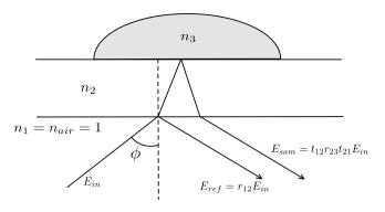
Figure 6. Ray schematic of the terahertz radiation path.
