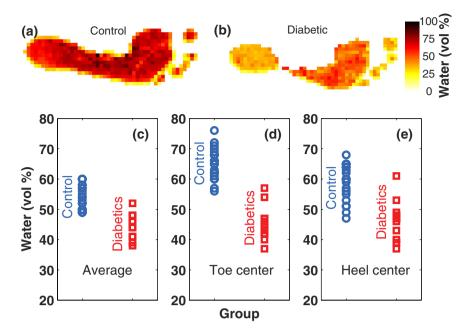
**Figure 2.** (a) Terahertz image of a typical member of the control group. (b) Terahertz image of a typical member of the diabetic group. Volumetric fraction of water for control group members and diabetics (c) averaged over the foot sole, (d) at the center of the greater toe and (e) at the center of the heel. Each point represents a subject.
