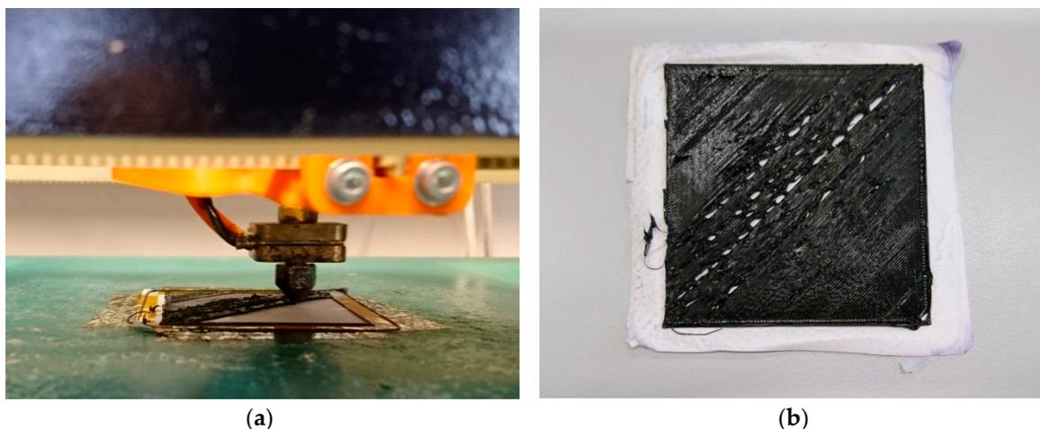
**Figure 3.** 3D printing squares of dimensions 40 mm × 40 mm on nanofiber mats previously dipped in soap water: (a) rough surface for a too large distance between nanofiber mat and printing nozzle; (b) 3D printed layer with uneven surface and even several not closed areas near the diagonal, i.e., along the longest lines, due to a too large distance between nozzle and nanofiber mat.
