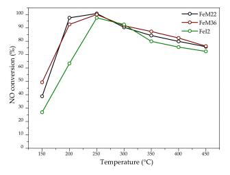
Figure 6. NO conversion obtained for the investigated one-pot synthesized Fe-MWW zeolites.
