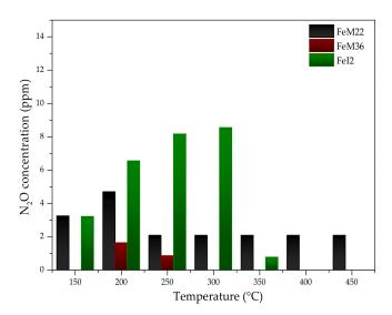
**Figure 7.** Concentration of  $N_2O$  in the gas mixture during  $NH_3$ -SCR catalytic tests conducted over Fe-MWW zeolites.
