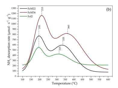
Figure 3. NH<sub>3</sub>-TPD profiles obtained for (a) pristine MWW zeolites; (b) iron-modified MWW zeolites.
