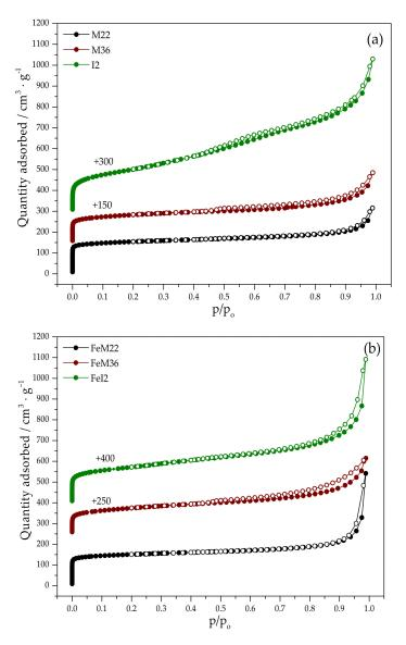
**Figure 2.** N<sub>2</sub> sorption isotherms obtained for the investigated materials: (a) pristine MWW zeolites; (b) iron-modified MWW zeolites.
