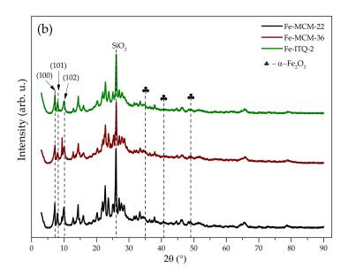
**Figure 1.** XRD patterns of the investigated materials: (a) MCM-22 (P) and its pristine derivatives in  $2\theta$  range of 2–40°; (b) iron-modified layered zeolites in  $2\theta$  range of 3–90°.
