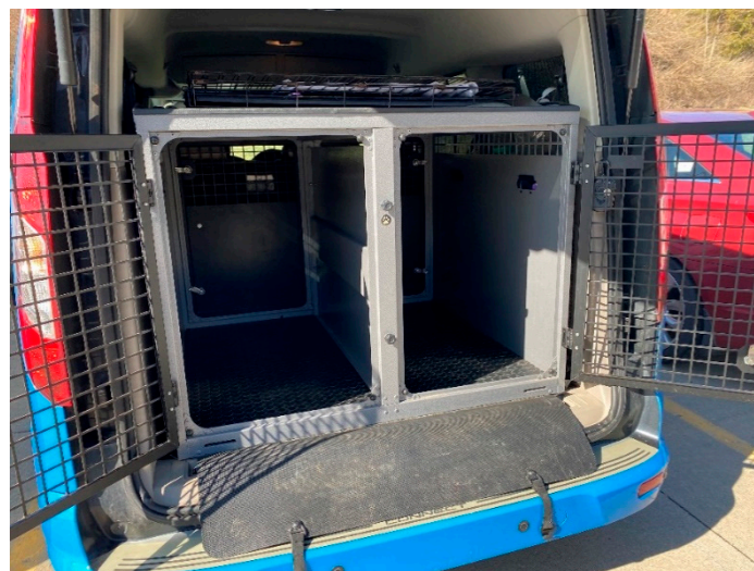
Figure 2. Cargo van with dual crate system and removable center divider.
