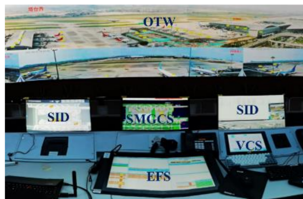
Figure 2. The layout of the digital tower module with a large LED panoramic screen.
