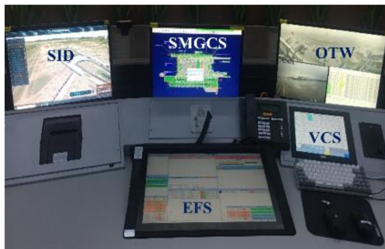
Figure 3. The layout of the digital tower module with a small LCD panoramic screen.
