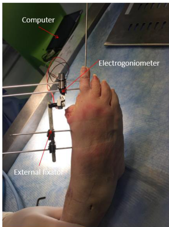
Fig. 11 Electro-goniometer for range of motion measurement
