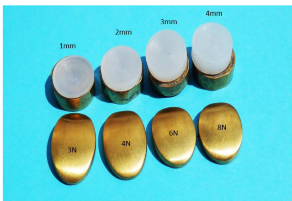
Fig. 14 The four implants each with the respective compressive forces as well as the sizes after completing 5,000,000 cycles at physiological forces
