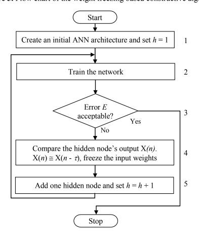
Figure 3. Flow chart of the weight freezing based constructive algorithm.
