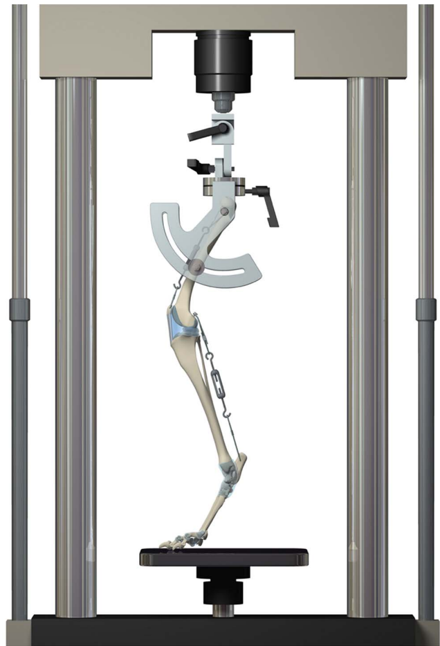
Figure 1. Schematic illustration of the prepared specimen mounted to a materials testing machine. Stifle and hock angles of 135\pm 5^{\circ} were attained with the limb subjected to an axial load of 30% body weight.
