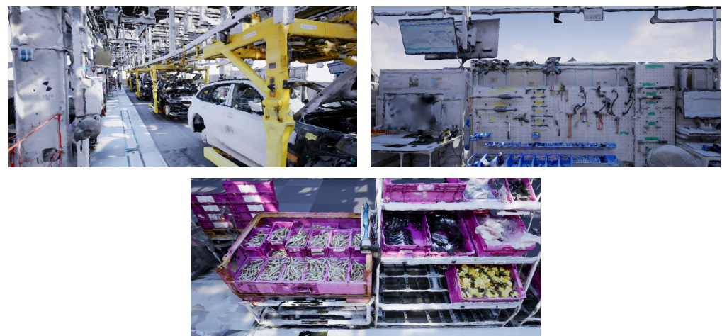
Figure 7. Visualization of the combined laser scan and photogrammetric point cloud as mesh.
