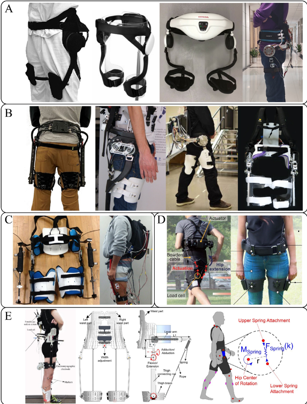
Figure 2. Hip exoskeleton with different actuators. (a) Motor with gear reducer (Shimada et al., 2009; Yasuhara et al., 2009; Buesing et al., 2015; Yang et al., 2021). (b) SEA (Giovacchini et al., 2015; Kang et al., 2018; Zhang et al., 2019a). (c) Pneumatic actuator (Young et al., 2017b; Thakur et al., 2018). (d) Motor with Bowden cable (Kim et al., 2019; Tricomi et al., 2022). (e) Passive (Zhou et al., 2021a,b).
