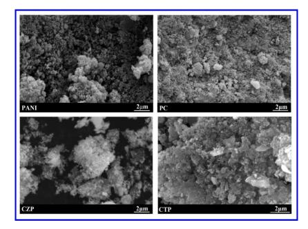
Figure 3. SEM images of PANI, PC, CZP and CTP nanocomposites.
