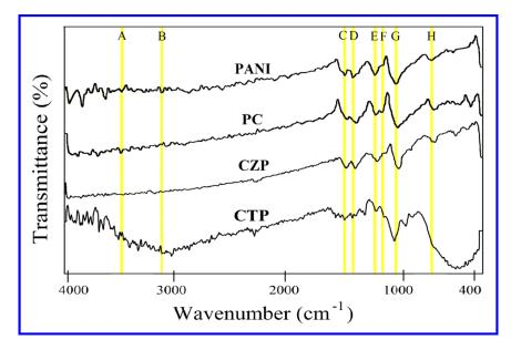
Figure 1. FTIR spectra of PANI. PC, CZP and CTP nanocomposites.
