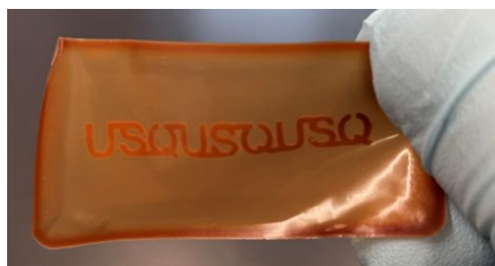
Figure S33. The digital image of as-prepared flexible AgNW/PU strain sensors.
