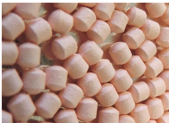
Figure 2. Coated ritonavir extrudate 2-mm particulate.
