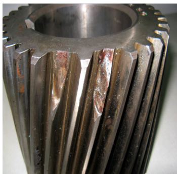
Figure 38. Collision of the gear Z5 on Shaft II of the bevel box.
