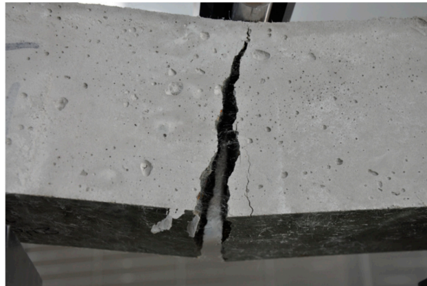
(a) PP fiber rupture
