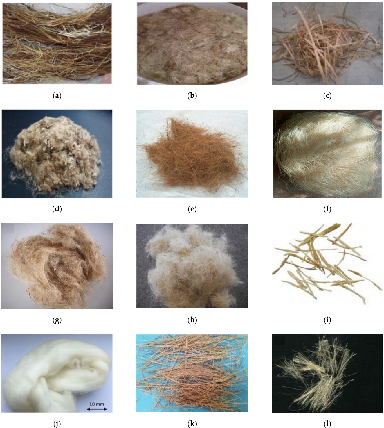
Figure 12. Natural polymer fibers used in CBMs. (a) Palm [144], (b) Hemp [145], (c) Banana [146], (d) Jute [147], (e) Coconut [148], (f) Abaca [149], (g) Kenaf [150], (h) Sisal [151], (i) Bagasse [152], (j) Wool [153], (k) Bamboo [154], (l) Flax fabric [155].
