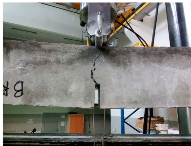
(b) Steel and glass fibers bridging
