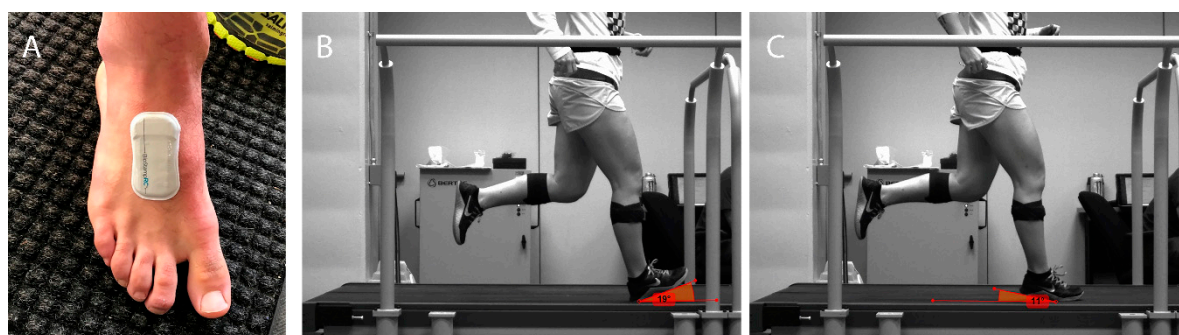
Figure 1. (A) BiostampRC sensor attached to the dorsal surface of the foot to determine sensor based foot strike angle ( FSA_{\text{SENSOR}} ) and foot strike classification ( FSC_{\text{SENSOR}} ). (B,C) View from camera showing the participant running on treadmill. This view was used by human raters to determine the foot strike angle from the video ( FSA_{\text{VIDEO}} ) and the foot strike classification from video ( FSC_{\text{VIDEO}} ). The image on the left (B) shows an example of FSA_{\text{VIDEO}} = 19^\circ and FSC_{\text{VIDEO}} = \text{rearfoot (RF)} . On the right (C) is an example of FSA_{\text{VIDEO}} = -11^\circ and FSC_{\text{VIDEO}} = \text{forefoot (FF)} .
