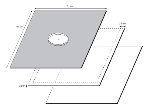
**Figure 1.** Tunneling arena ( $61 \times 61$  cm) constructed of two sheets of transparent Plexiglas ( $61.0 \times 61.0$  cm) separated by four Plexiglas strips ( $61.0 \times 2.5 \times 0.3$  cm) affixed to the outer margins with screws. One access hole (6.5 cm diameter) was drilled at the center of the top sheet and fitted with an ant release chamber.
