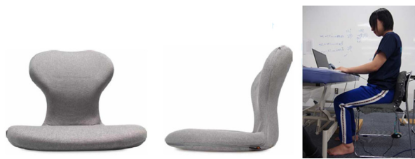
Fig. 1. Front and side views of the developed chair with active lumbar support Right figure: Experiment environment
