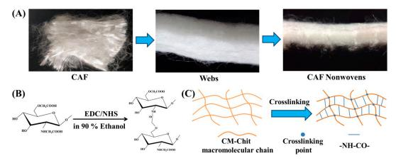
**Figure 1.** Structure changes in the fabrication of composite wound dressings. (**A**) The structure of CAF, webs and needle-punched nonwovens. (**B**) The chemical structure and (**C**) the macromolecular chains structure of CM-Chit during crosslinking.
