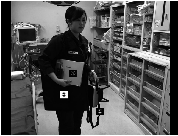
Fig. 1. CALNEO Xair portable X-ray system, developed by Fuji-film (Tokyo, Japan), being carried by a nurse. (1) X-ray radiating apparatus. (2) Special cassette. (3) Notebook-type personal computer.
