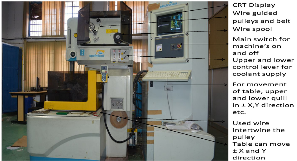
Fig. 1. Experimental setup of WEDM machine.
