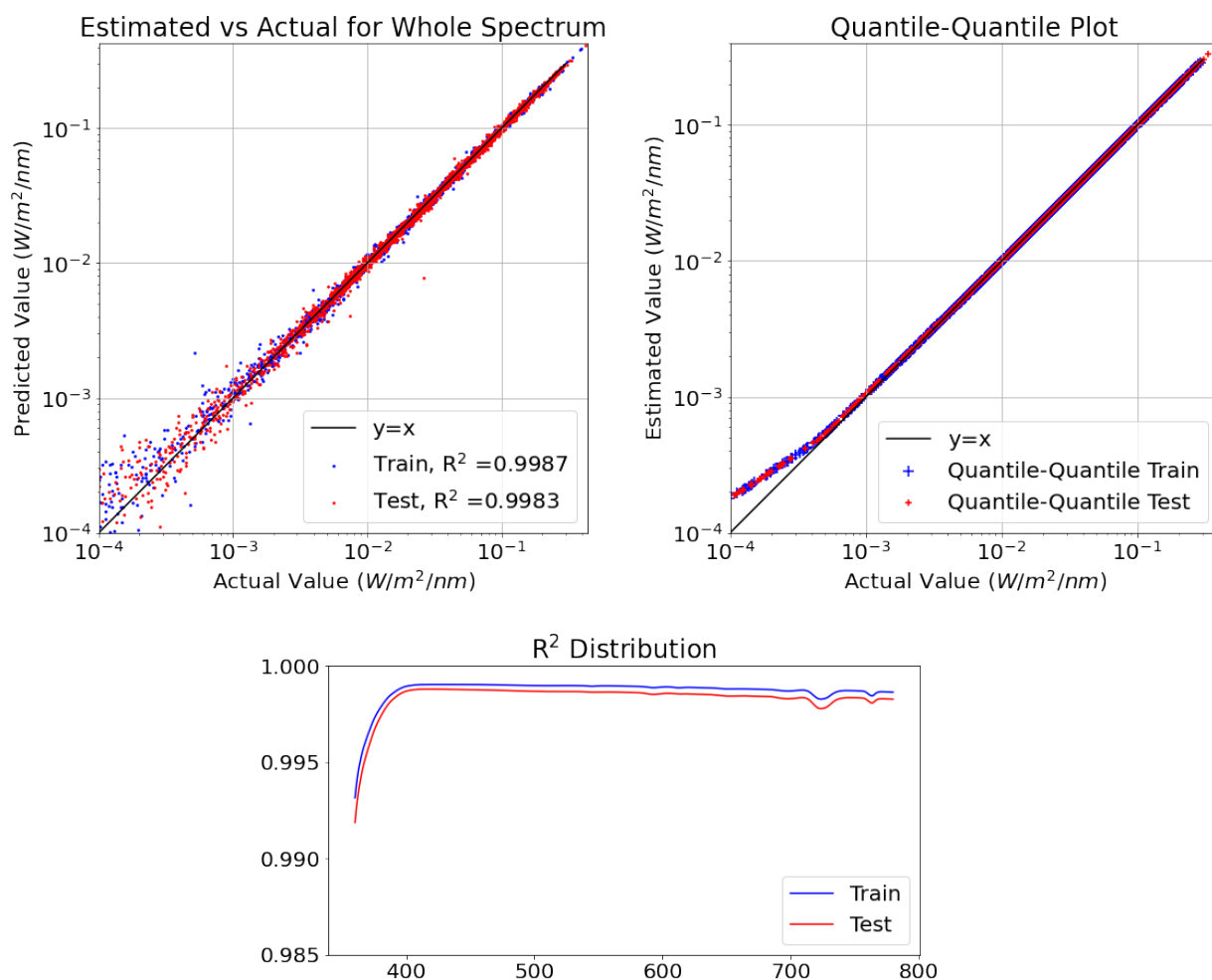
Figure 7. Whole spectrum model performance and the R2 scores on different wavelengths.
