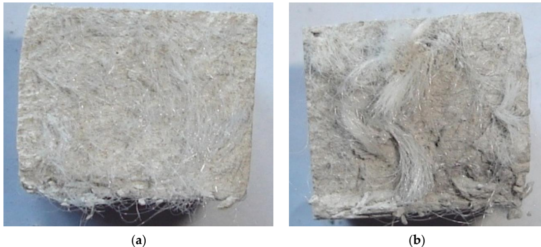
Figure 9. Uniform (a) and uneven (b) distribution of polyamide fiber in hardened GCB-FA specimens.
