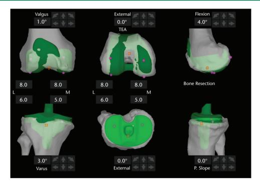
**Fig. 4** Operative plan for a robotic-assisted, kinematically aligned TKA. Note that the implant alignment is based on symmetrical 8 mm distal and posterior resections of the femoral condyles. The tibial resection is aligned to the native proximal tibial joint line, taking into consideration 1mm of asymmetrical bone loss from osteoarthritis.
