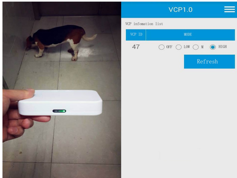
Figure 4. Activity of capsules can be detected and adjusted by configurator and configurator-matched App externally.
