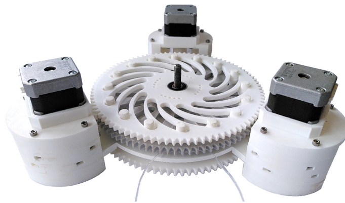
Figure 19. Assembled pump with all gears and motors.
