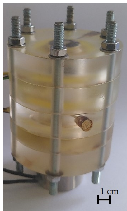
Figure 12. Assembled decanter consisting of a total of 5 acrylic glass modules.
