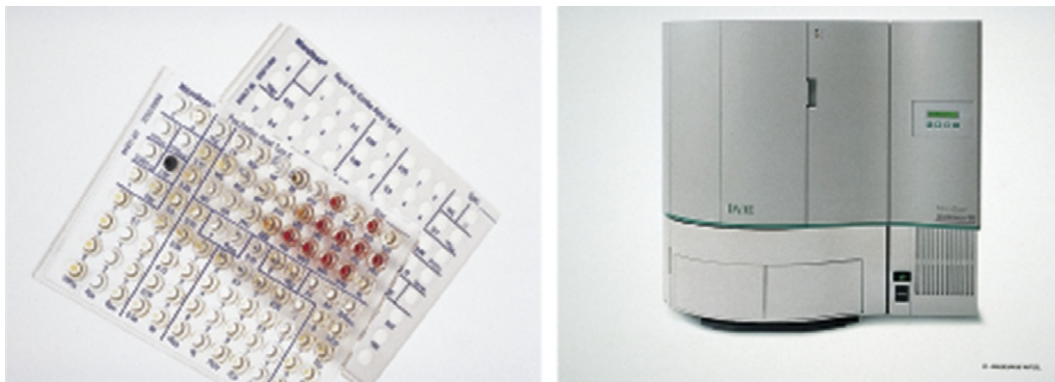
Figure 43 Microbroth tray format (a) used with the MicroScan WalkAway instrument (b) for automated incubation, reading, and interpretation of antimicrobial susceptibility tests. Courtesy Dade International, Sacramento, CA. Reprinted from Figure 12-14 of Forbes, B.A., Sahn, D.F., Weissfeld, A.S., 2007. Bailey & Scott's Diagnostic Microbiology. Mosby Elsevier, St. Louis, with permission from Elsevier.
